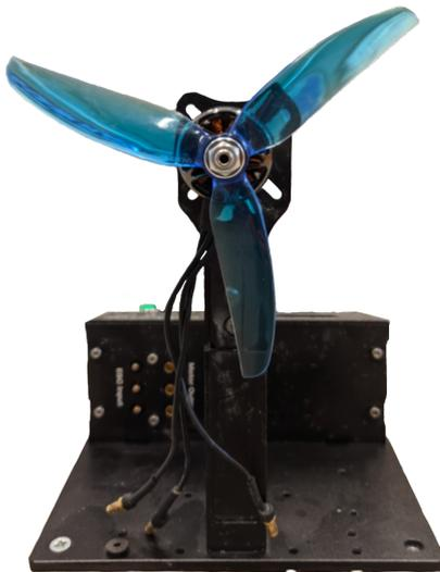
Figure 8 – Motor *EMax ECO II 2207 2400KV* with propellers of 5" radius, 4.3" pitch and 3 blades (5x4.3x3) mounted in the thrust bench used for the static thrust tests.
