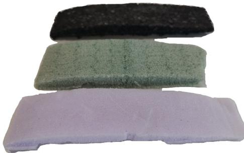
Figure 10 – Wing sample for foam testing - From back to front EPP, PVC and XPS foam.
